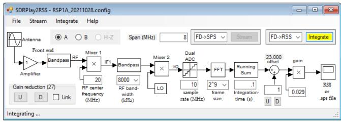
Illustration 1: SDRPlay2RSS window showing the signal path of the radio and software with adjustments along the path
